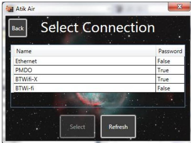
The top option will always be 'Ethernet' and is the direct Ethernet connection to the Raspberry Pi. The others will be any wifi sources in range of the Raspberry Pi. The right column indicates whether or not the connection needs a password.
