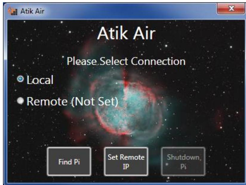
*You will see two options 'Local' and 'Remote'. Local will look for cameras connected to your PC. Remote will look for cameras connected to the Raspberry Pi. The first time you see this screen, Remote will say 'Not Set'. Before you can use the cameras connected to the Raspberry Pi, you will need to set it up.*
